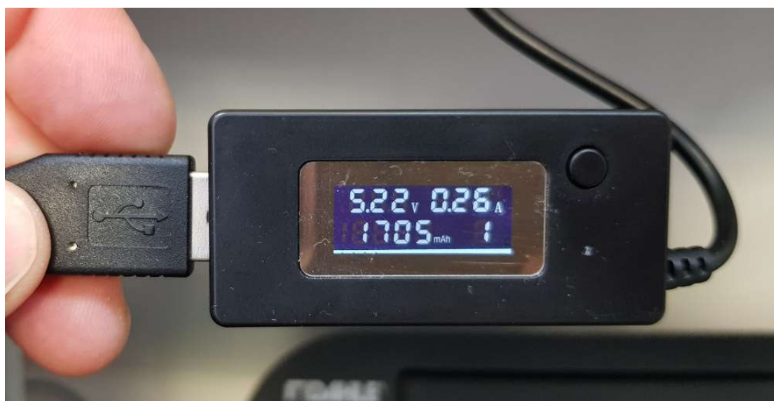
Figure 6: Measuring device for loading the IR thermography camera
