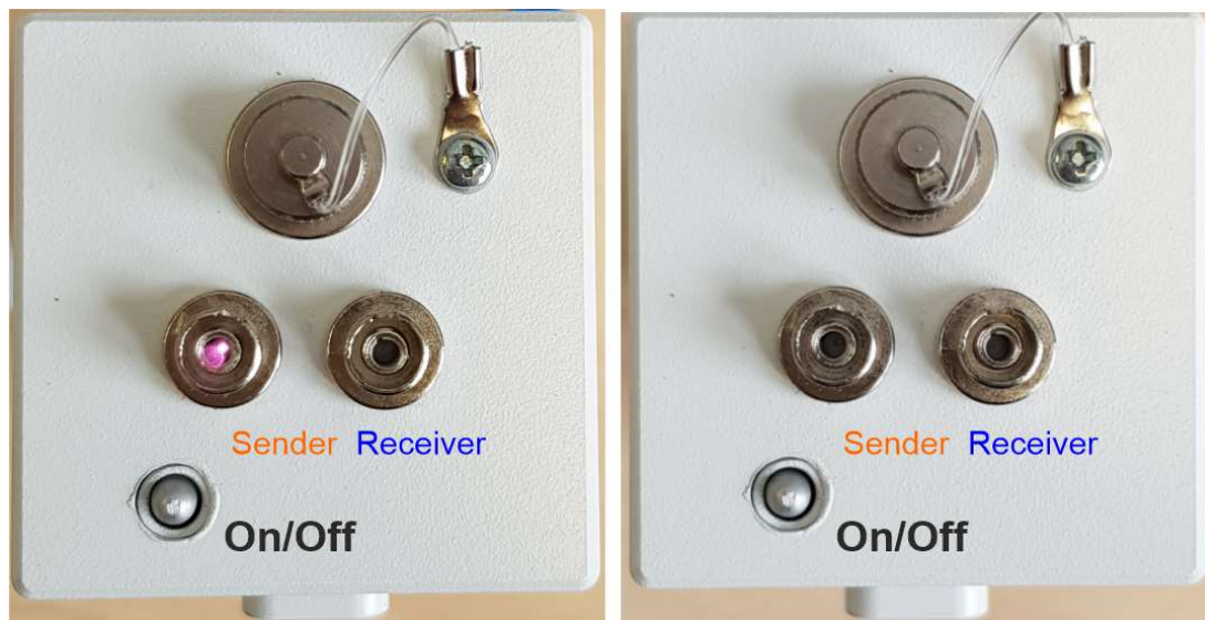
Figure 4: State of the IR thermography camera (left ON, right OFF).
